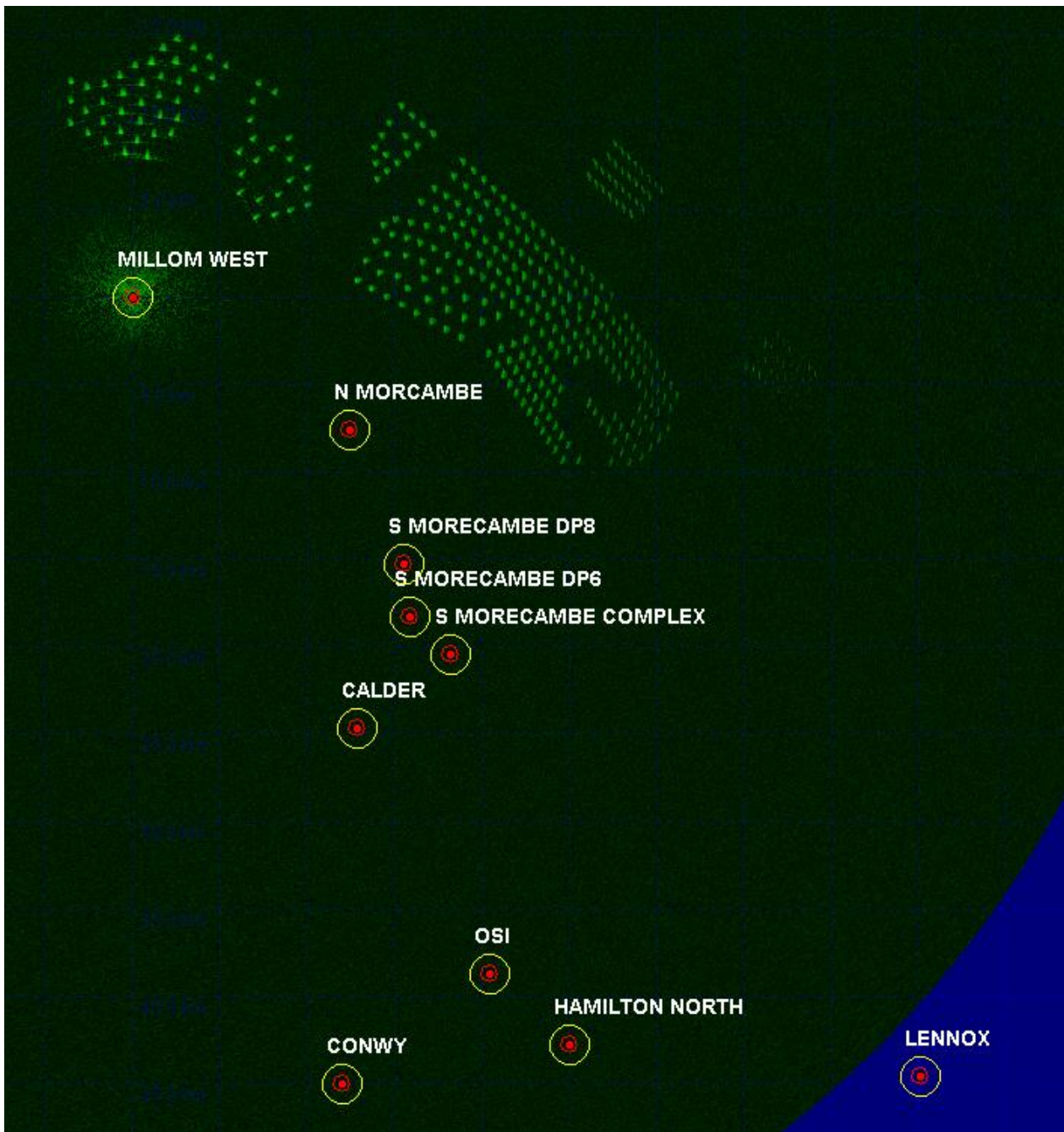
Figure 4.7: Harbour Energy's Millom West platform REWS clutter map showing returns from the wind turbines and sea clutter.
