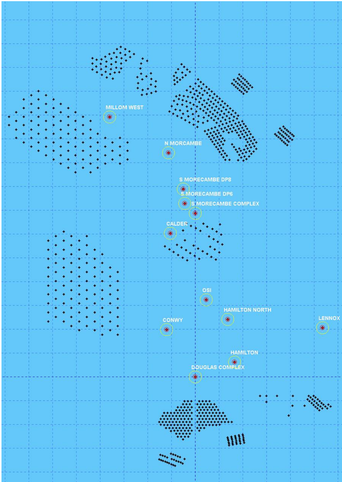
Figure 4.30: Modelled cumulative layout of the Morecambe Generation Assets with Mona Offshore Wind Project and Morgan Generation Assets showing the indicative location of the wind turbines and the location of oil and gas platforms in the region.
