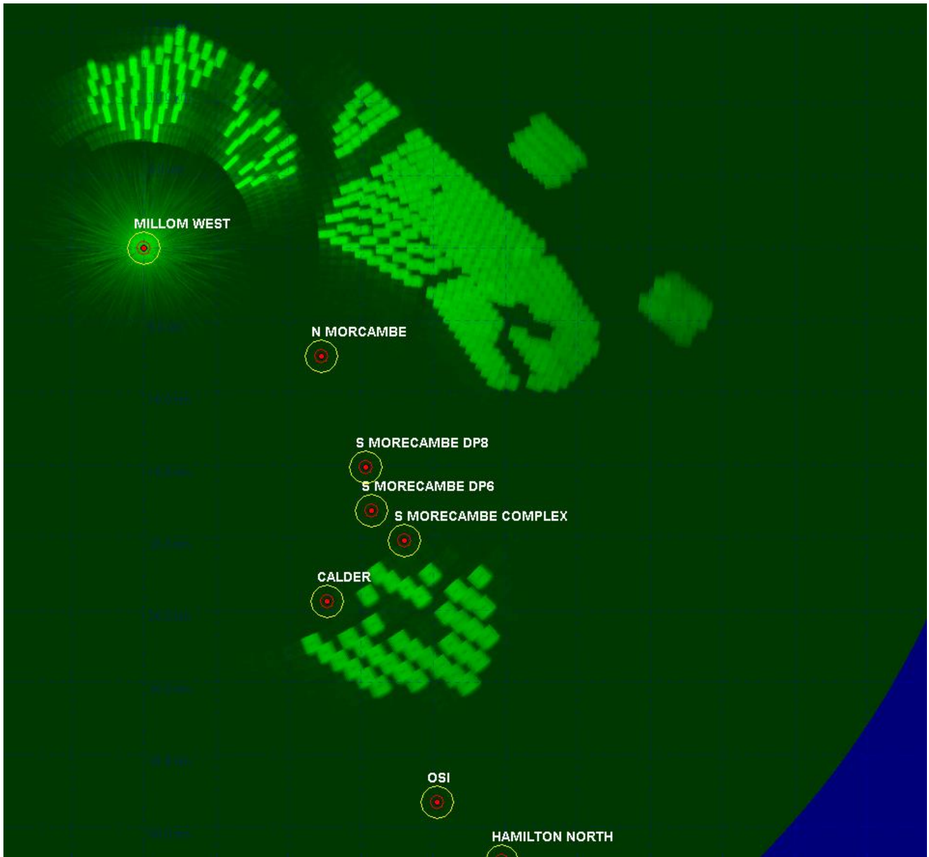
Figure 4.21: Harbour Energy’s Millom West platform REWS detection threshold over the Morecambe Generation Assets Array Area.
