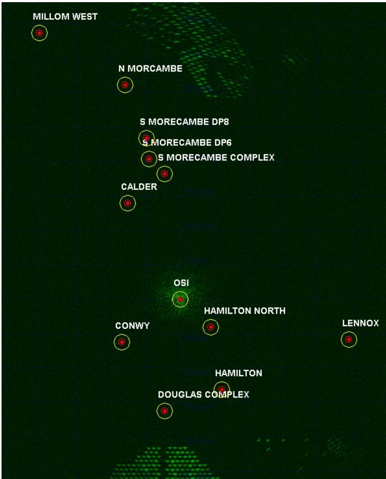
Figure 4.10: ENI Energy's OSI REWS clutter map showing returns from the wind turbines and sea clutter.
