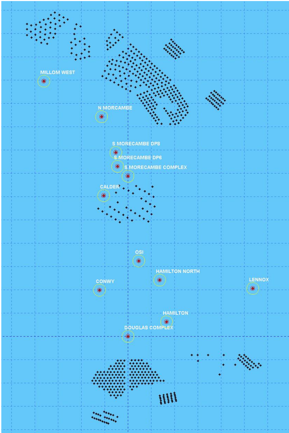
Figure 4.16: Modelled layout of the Morecambe Generation Assets showing the indicative location of the wind turbines and the location of oil and gas platforms in the region.
