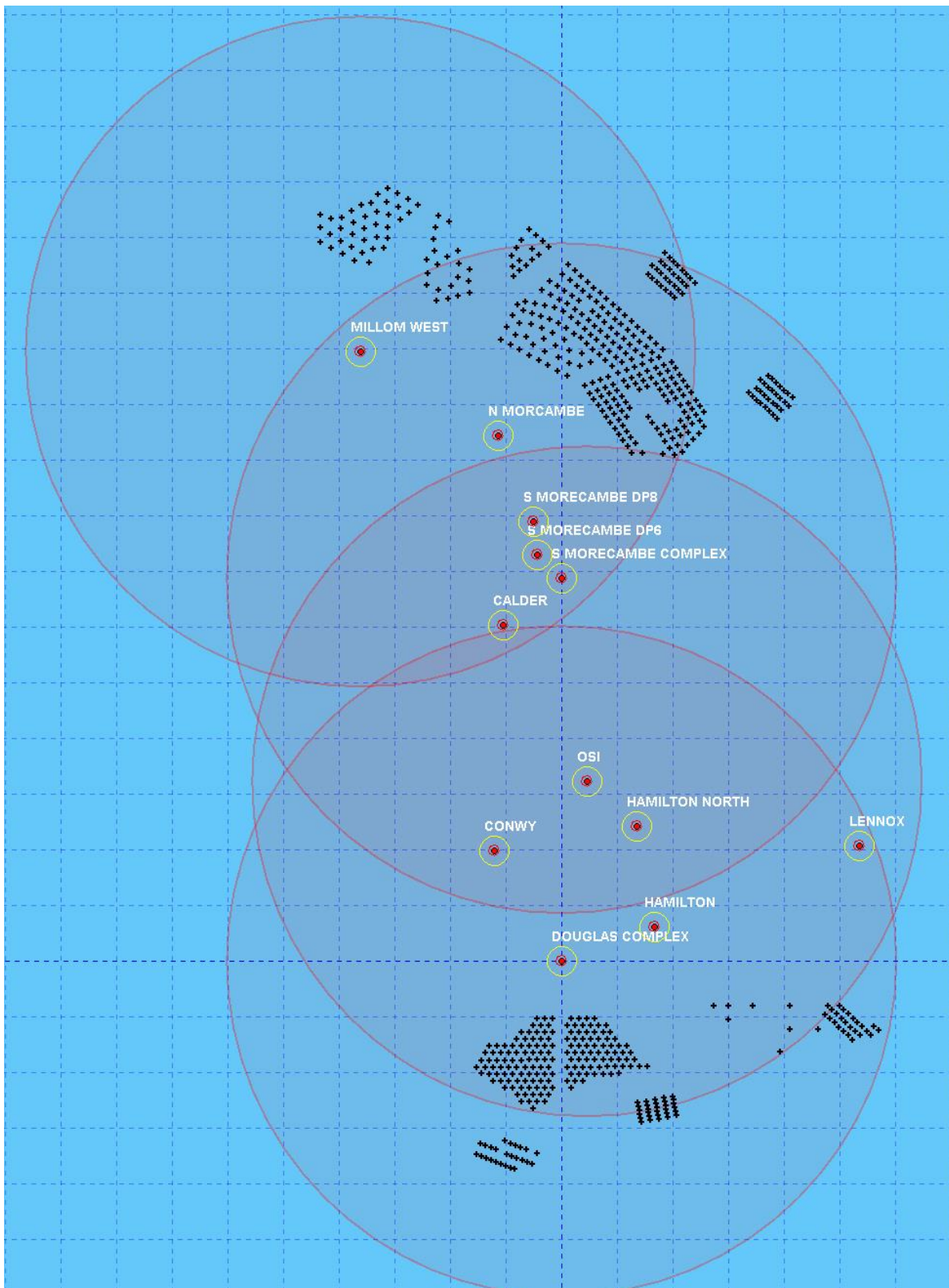
Figure 4.1: Modelled layout of the base case scenario showing the location of the existing windfarms and the coverage of the REWS in the region.
